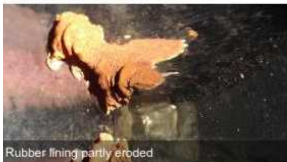
Dredger KSB pump, cavitation damage
