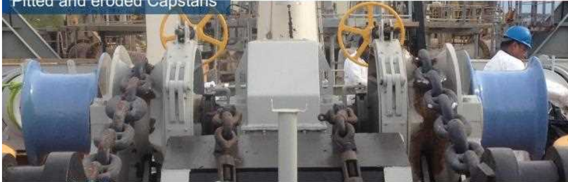
Pitted and eroded Capstans
