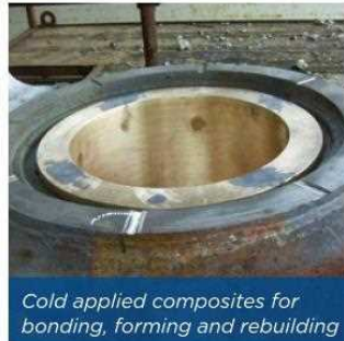
100% solids chocking compounds for installation of equipment
