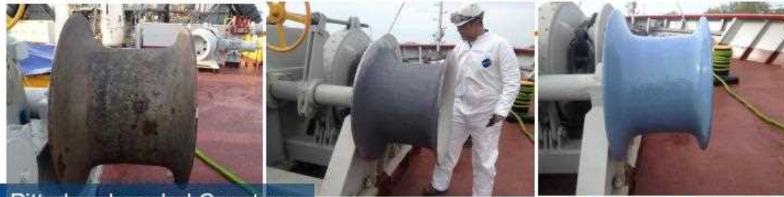
Pitted and eroded Capstans
